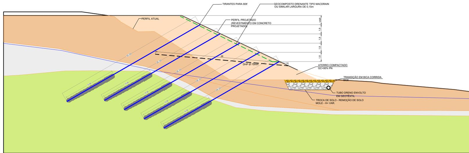
DETALHE DA SAÍDA DO GEOCOMPOSTO DRENANTE SEM ESCALA
